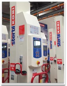
Now, Stertil-Koni is bringing this technology to its more economically priced wired mobile column lifts, which also showcase the best in heavy duty hydraulic lifting, but use interconnecting communication wires rather than wireless connectivity.
